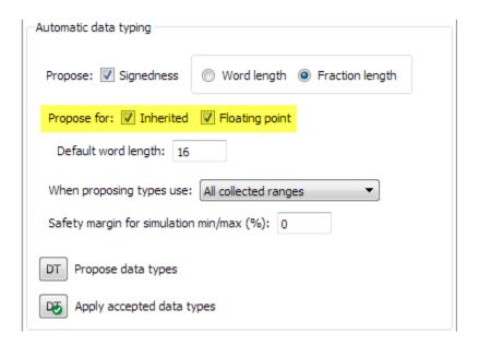
By default, the **Inherited** and **Floating point** check boxes are selected. If you clear the **Inherited** or **Floating point** check boxes, the Fixed-Point Tool will not propose a fixed-point data type for results that use an inherited or floating-point data type respectively.
