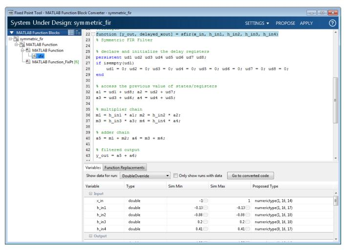
Once you are satisfied with the proposed data types, click **Apply** to have the tool automatically generate a variant subsystem. The variant subsystem contains the original floating-point version of the MATLAB function block, and a fixed-point version of the block. You can refine the conversion by modifying the original floating-point MATLAB code. The fixed-point variant will automatically update after reconverting the block.
